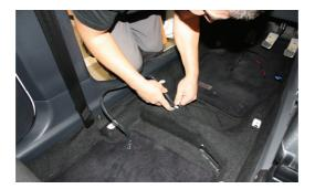
**(2)** Re-install the seat; if it has airbags, reconnect its cables. **CAUTION!** It is forbidden to connect the airbag cables in a car under power. Connect the cables managed in the previous steps.
