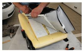
8 Remove the seat cover from the back cushion, and install the heating panels as per the instructions above.
