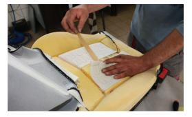
6 Drill a hole into the cushion, then lace through the wiring harness.
