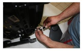
Place the wiring harness under the floor carpet. Connect the positive (red) and negative (black) cables to the car's electronic system via a fuse. It is recommended to connect to a point which will be powered after the ignition. Thus the heating cannot discharge the battery, even if you forget to turn it off after stopping the vehicle.
