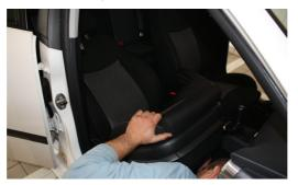
**3** Remove those plastic covers which may interfere with the removal of the seat cover. If it is possible, separate the bottom cushion and the back cushion.
