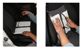
2 Remove the seat from the vehicle. If there is airbag in the seat, turn off the car then wait for at least 30 minutes before proceeding. Never turn on the car during the installation. Try not to disconnect the airbag's connectors if possible.
