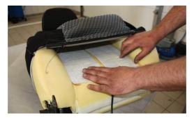
**9** The wiring harness is supposedly channelled through one of the sides. Re-install the seat cover and the plastic covers.
