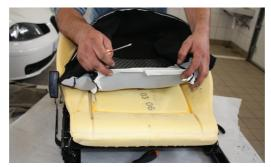
S Place the heating panels onto the bottom cushion and fix it with two-sided adhesive tape. The wiring of the bottom heating panels is black, while the back heating panels' is yellow-red-black. The metal barces of the seat cover must not situated on the heating panels, because of the danger of short circuit and fire.
