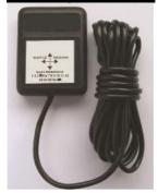
Futures No mechanical elements No settings Dimension 41x52x12 mm Power: 5-16 VDC or 17-30 VDC Power consumption: 1,3 mA (at 12 V) Time of signal: 4 s , or 25 s when loop is cut (loop is inside) Sensitivity: change angel for 0,9 degree Time to setup a new position: max 45 s **Install in horizontal position only**
