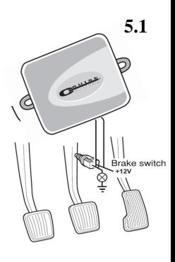
**Digital Brake Link connection**: for vehicles with a digital brake link connect the BROWN wire to a permanent ignition switched feed (+15) at another location (for example fuse-box).
