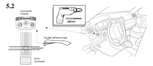
**A** NOTE: Place the 8-pole connector on the wiring harness after the command module is placed on its location and after the wiring harness to routed to the Cruise Control ECU.
